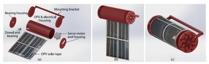
Figure 7: PV-Pix prototype 2 – *FabricOn*. This prototype is constructed using a commercially available flexible organic photovoltaic (OPV) solar-cell, a servo motor and a series of 3D-printed and laser-cut housings (a), and rolls up or down to change between the (b) open and (c) closed states. Note that as in Fig. 6 we use rendered diagrams of the prototype for clarity here, and the accompanying video figure shows working examples of the actual prototype in use.
