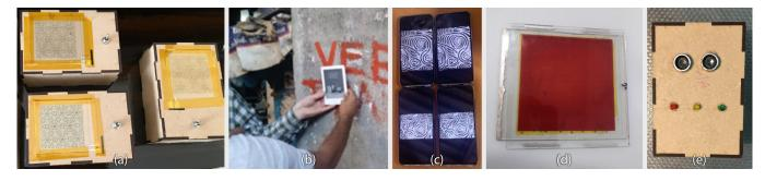
Figure 3: The technology probes we used in the community workshop in Dharavi. From left to right: (a) electrochromic displays, (b) E Ink displays, (c) connected phone array, (d) dye-sensitised solar cell (DSSC), (e) proximity sensor with LEDs.
